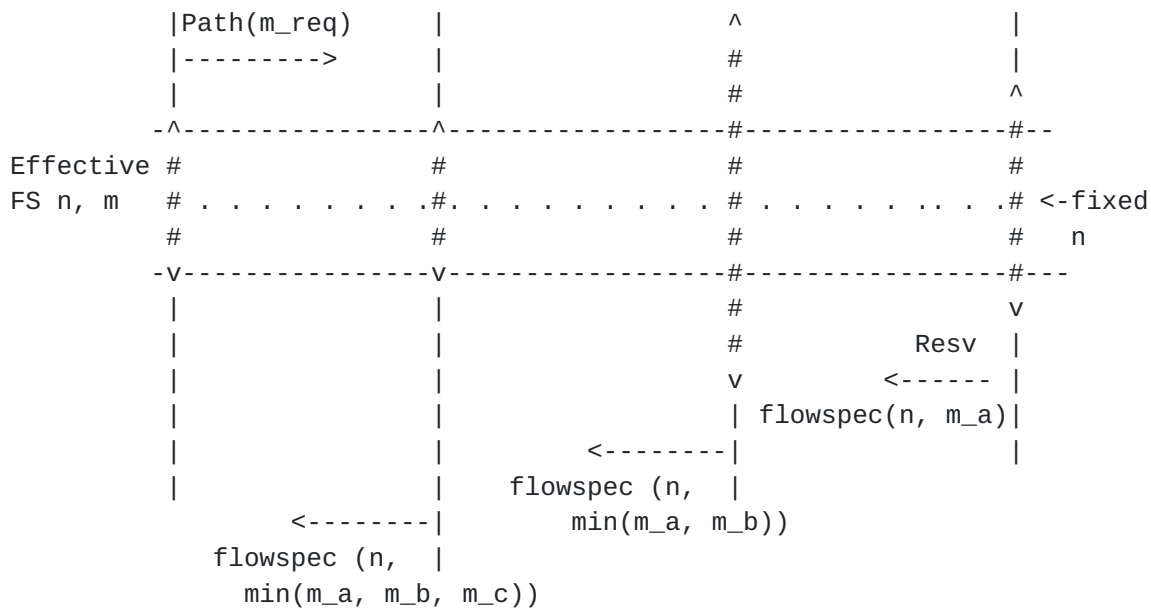
Figure 15: Distributed allocation with different m and same n
