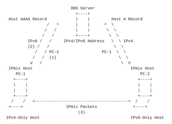
Step-1 ==> PC-1 needs to communicate with PC-2, it sends a query to the DNS server (with either IPv4 or IPv6 address) to resolve the hostname PC-2.
