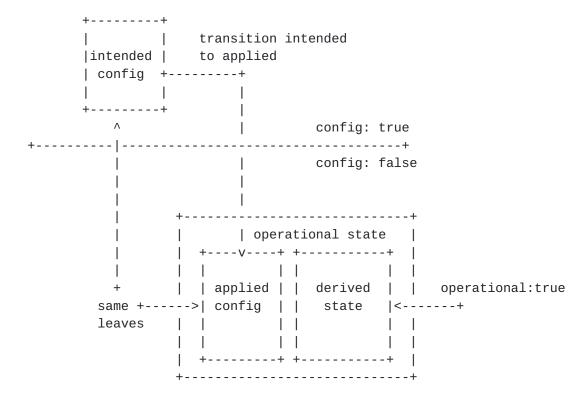
The relationship between intended and applied configuration, and derived state. The combination of the applied and derived state is referred to as the operational state.
