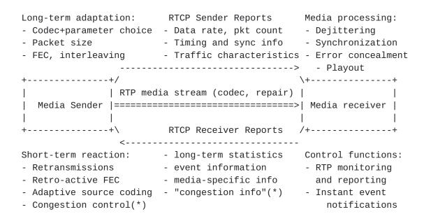
(\*) RTCP feedback is insufficient for TCP-Friendly congestion control purposes due to the infrequent nature of reporting (which should be in the order of once per RTT), but can still be used to adapt to the available bandwidth on slower timescales.
