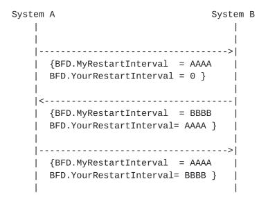
The initial BFD packet exchange between local system and remote system will have the exchanged values for the "My Restart Interval" or O. The "Your Restart Interval" will reflect the value received in My Restart Interval" from the corresponding remote system, or be Zero if that value is not set (value of 0).
