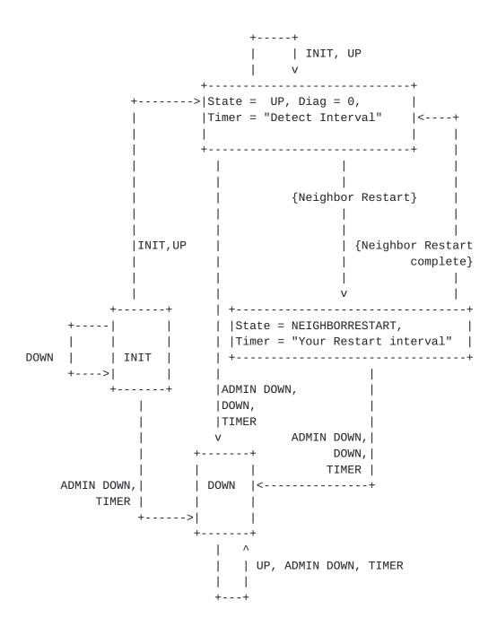
Note1: This state diagram holds only for BFD with GR extension as described in this document, which implies that "your Restart Interval" has a value greater than the Detection time value of the established session. This state machine must not be implemented.
