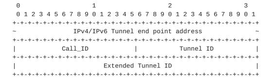
IPv4/IPv6 Tunnel End Point Address: 32 bits/128 bits (see [RFC3209])
