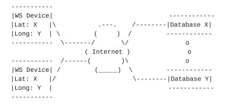
An example high-level architecture of the devices and white space databases is shown in the figure below:
