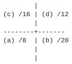
The figure above illustrates a router with 4 interfaces, a, b, c, d, each which is aggregating routes with the respective prefix. If a SM data packet arrives on interface (b) carrying a "scope mask(len)" of 12, it is forwarded only over interface (c) and (d).
