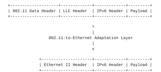
The Receiver and Transmitter Address fields in the 802.11 Data Header contain the same values as the Destination and the Source Address fields in the Ethernet II Header, respectively. The value of the Type field in the LLC Header is the same as the value of the Type field in the Ethernet II Header. The other fields in the Data and LLC Headers are not used by the IPv6 stack.
