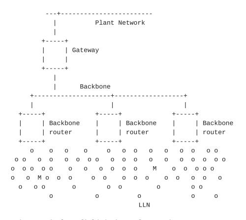
o : stationary wireless field device, often acting as an LLN routerM : mobile wireless device
