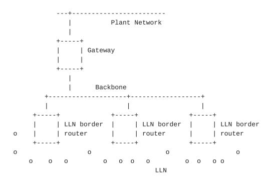
o : stationary wireless field device, seldom acting as an LLN router
