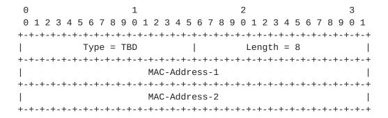
Length: In bytes for the value part of the Type/Length/Value encoding. The MAC-Address identifier will be 8 bytes long.
