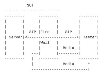
Figure 4. SIP Test Topology with Media through Firewall
