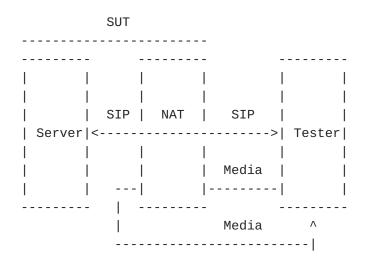
Figure 5. SIP Test Topology with Media through NAT Device
