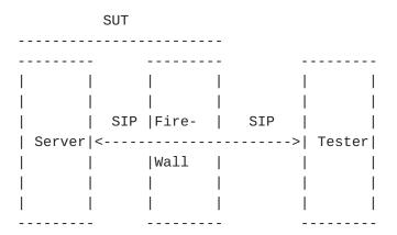
Figure 2. SIP Test Topology with Firewall
