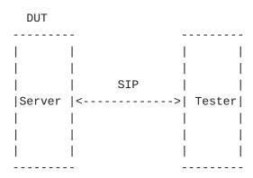
Figure 1. Basic SIP Test Topology
