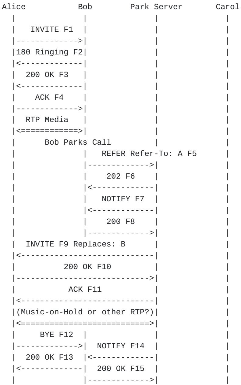
The URI `<sips:park-server@example.com;orbit=1234>` is used instead of directing the request to the URI `<sips:park@server.example.com>`. The addition of the orbit parameter effectively tags the parked call with a short memorable code entered by the user.
