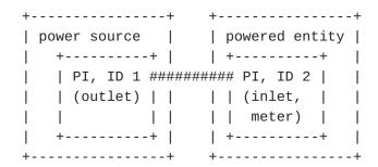
This figure extends the PSU layer of <u>Figure 3</u> by power interfaces. The power source has a single power interface in outlet mode connected to a power supply lime that connects it to the power interface of the powered entity in inlet mode. The corresponding PSU layer model of the topology in <u>Figure 7</u> is shown by <u>Figure 8</u>.
