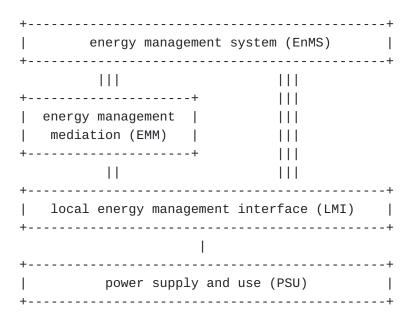
At the power supply and use (PSU) layer electrical objects (powered entities) are physically connected by power supply lines. Their connections constitute an electric supply and metering topology. The local energy management interface (LMI) layer provides a set of functions for monitoring and controlling individual powered entities.
