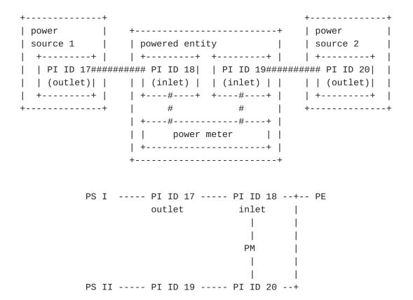
A power meter can cover any mixture of inlets and outlets and simply reports the sum. As an example, see the model of a the dual role PE and PS from <a href="Figure 13">Figure 13</a> extended by a power meter attached to all PIs in <a href="Figure 16">Figure 16</a>.
