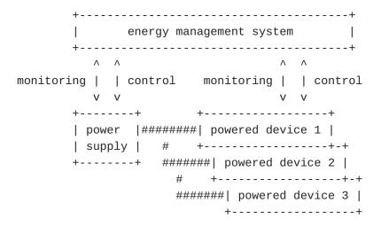
With this list, the single status value has clear meaning and is the sum of all powered devices. Control functions are limited by the fact that supply for the concerned devices can only be switched on or off for all of them at once. Individual control at the supply is not possible.
