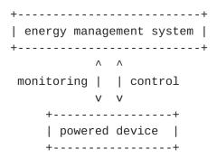
The device may have local energy control mechanisms, for example putting itself into a sleep mode when appropriate, and it may receive energy control commands for similar purposes from a management system. Information reported from a powered device to the energy management system includes at least the power state of the device (on, sleep, off, etc.).
