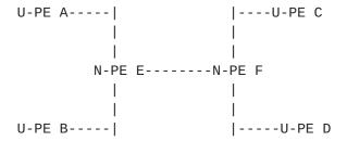
where the four U-PEs are in a common VPLS. In distributed VPLS, there will be three PWs from A to E. Call these A-E/1, A-E/2, and A-E/3. There will be two PWs from E to F. Call these E-F/1 and E-F/2. And there will be three more PWs, one from E to B (E-B/1), one from F to C (F-C/1), and one from F to D (F-D/1).
