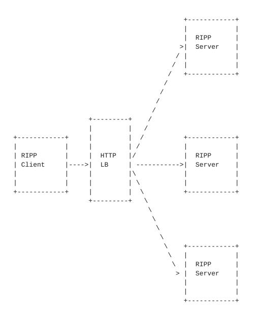
Since both the trunk provider and trunk consumer implement the client and server roles, both entities will typically have a load balancer perhaps a server component, or a cloud-based service, used to receive incoming calls. This is not required, of course. It is worth restating that this load balancer is NOT specific to RIPP - it is any off-the-shelf HTTP load balancer which supports HTTP/3. No specific support for RIPP is required. RIPP is just a usage of HTTP.
