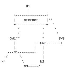
Figure 1: MANET interconnected to an external network
