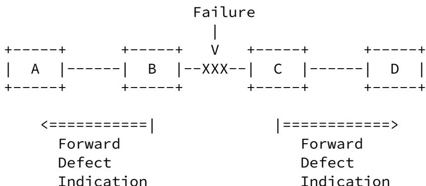
Figure 3: Forward Defect Indication
