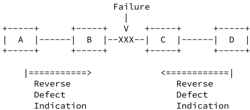
Figure 4: Reverse Defect Indication
