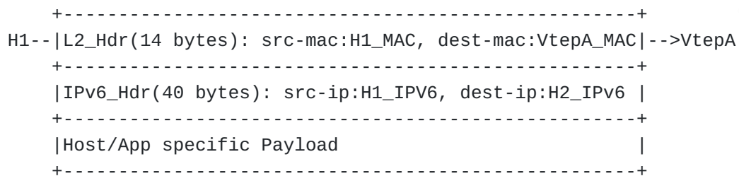
Figure 2a. Packet P1 sent by host H1 to host H2
