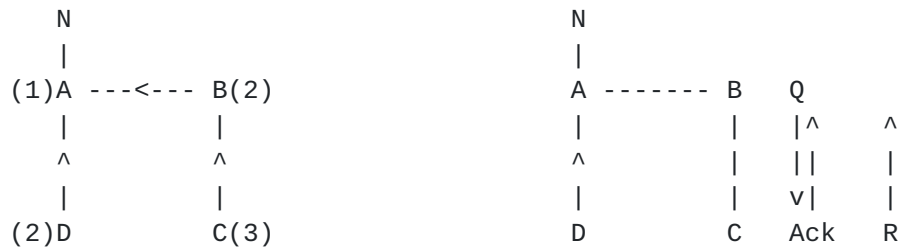
Figure 4 No Feasible Successors when link between A and B fails
