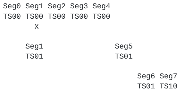
Figure 4: timestamp for spurious retransmit detection
