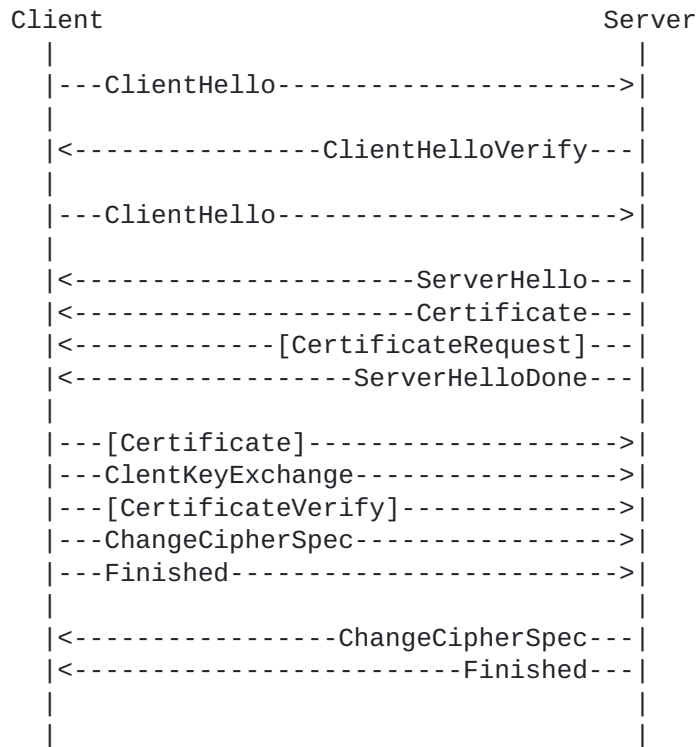
Figure 2: Message Flow of Two-way Authentication Handshake for Class 2 Devices
