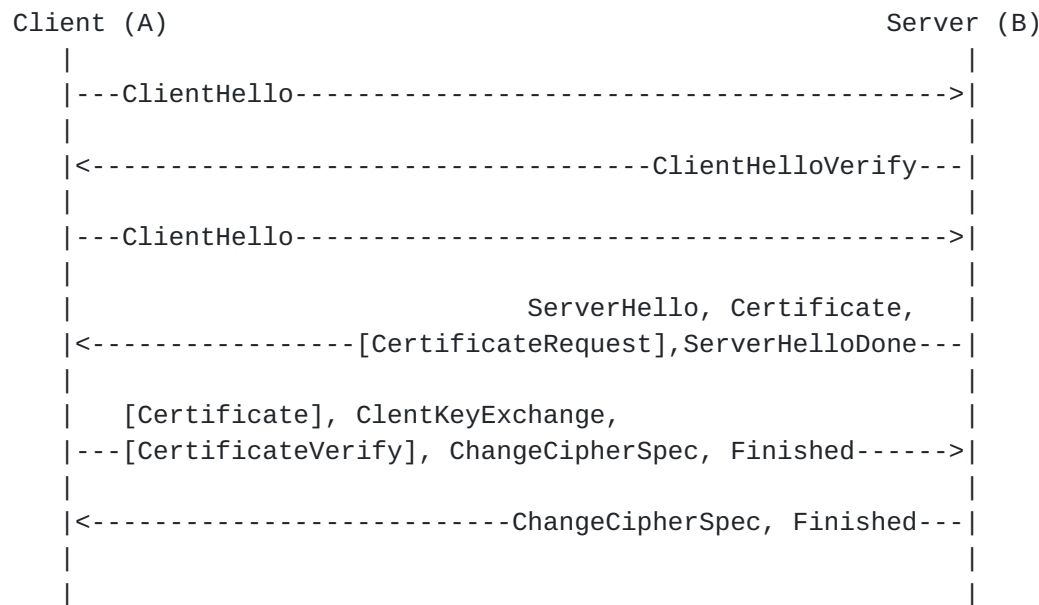
Figure 2: Message Flow of Two-way Authentication Handshake for Class 2 Devices
