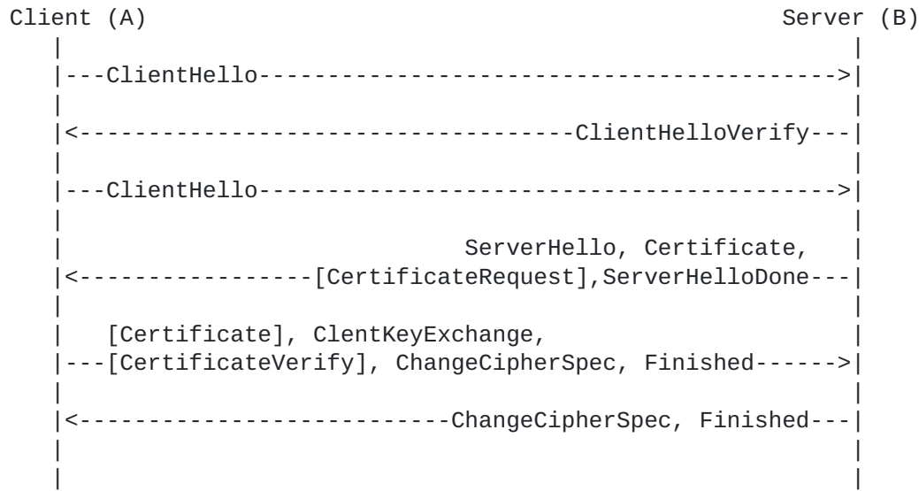
Figure 2: Message Flow of Two-way Authentication Handshake for Class 2 Devices
