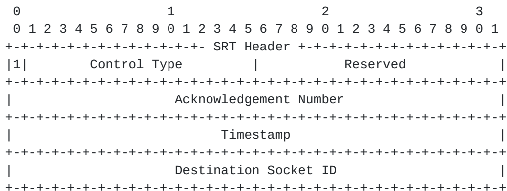
Figure 16: ACKACK control packet
