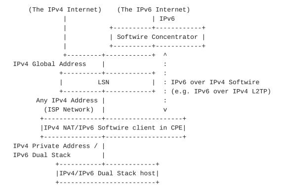
Step 3: Moving on to dual stack ISP provides dual stack access to CPE. A CPE uplink is now dual stack.
