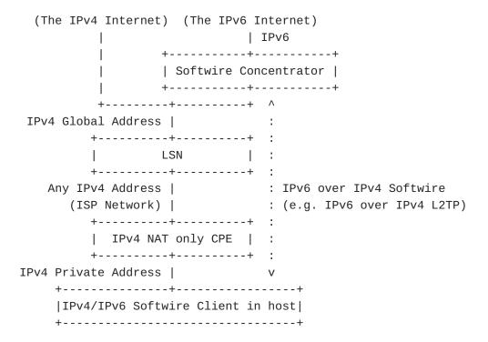
Step 2: Enabling softwire client in CPE A customer enables softwire client in CPE. A softwire client in CPE connects to the IPv6 internet via ISP's concentrator. A Customer's network is now dual stack.
