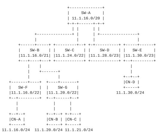
If a host in CN-A wants to send a packet to an address 11.1.21.116, CE router of CN-A forwards it to SW-F. SW-F finds the destination address of the packet to be outside of its domain and forwards the packet to its parent SW-B. SW-B finds that a port that has been configured with the matching destination address and forwards it to its child SW-G. Switch SW-G sends the packet to customer network CN-B.
