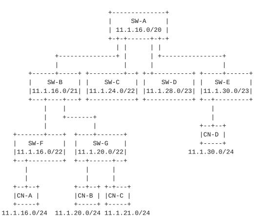
If a host in CN-A wants to send a packet to an address 11.1.21.116, CE router of CN-A forwards it to SW-F. SW-F finds the destination address of the packet to be outside of its domain and forwards the packet to its parent SW-B. SW-B finds that a port that has been configured with the matching destination address and forwards it to its child SW-G. Switch SW-G sends the packet to customer network CN-B.
