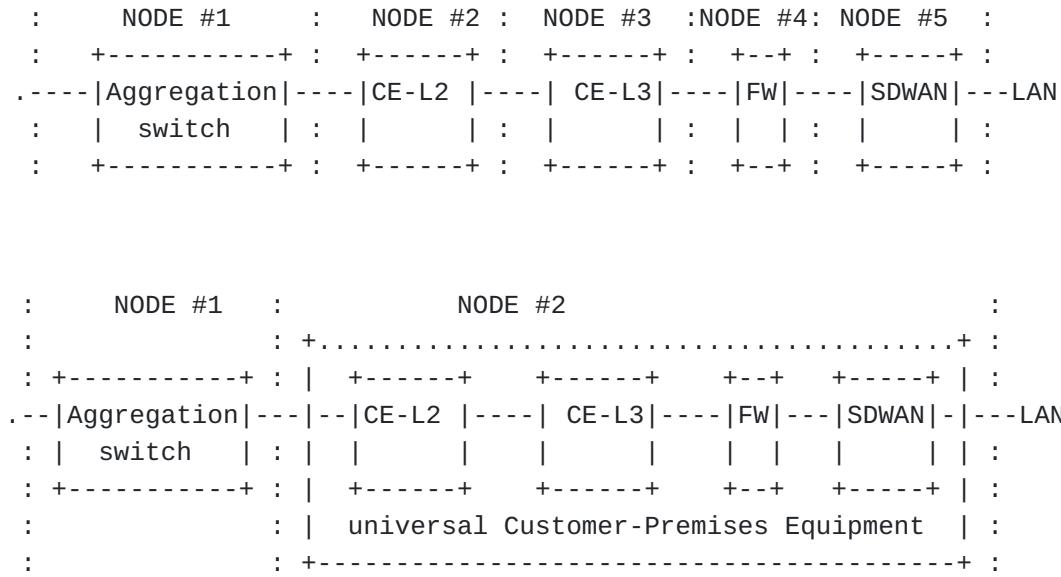
\*uCPE facilitates the interconnection between the Network Functions (NF) as interconnection between NF is performed via virtual links(that is part of the uCPE management). That means that no need to hire technician to cable the equipment, it could be done via orchestrator.
