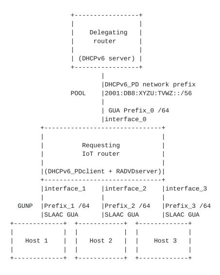
(In the above figure the scenario with 3 hosts connected to the Requesting IoT router is presented. Normally there are no number limitations of connected hosts.)
