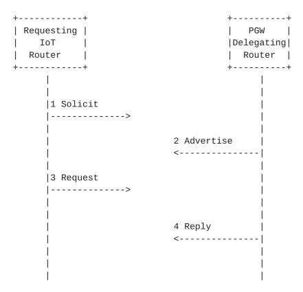
(In the above figure the full DHCPv6 message exchange mechanism between the ARM part of UE and PGW is presented.)
