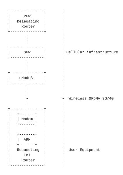
(The above figure descibes the model of the path followed by a DHCPv6 packet from IoT requesting router to the Delegating PGW router. The model is not a real infrastructure.)
