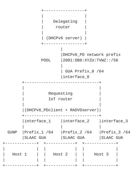
(In the above figure the scenario with 3 hosts connected to the Requesting IoT router is presented. Normally there are no number limitations of connected hosts.)
