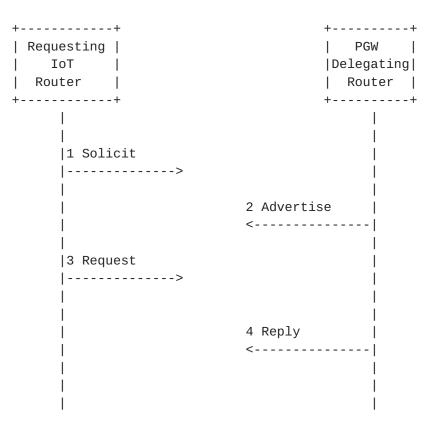
(In the above figure the full DHCPv6 message exchange mechanism between the ARM part of UE and PGW is presented.)
