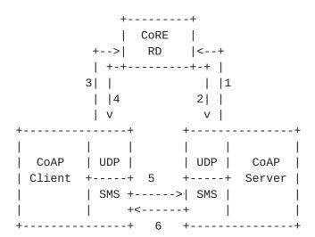
Figure 3: CoAP client interacting with RD to discover a server's SMSbased endpoint
