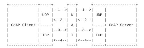
Figure 1: CoAP Client initially accesses CoAP Server over UDP and then switching to TCP
