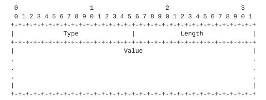
Types are defined below; Length is the length of the Value field in octets. The Value field depends on the Type; it is zero padded to align to a 4-octet boundary. TLVs may be nested within other TLVs, in which case the nested TLVs are called sub-TLVs. Sub-TLVs have independent types and MUST also be 4-octet aligned.
