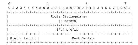
The Route Distinguisher (RD) is an 8-octet identifier; it does not contain any inherent information. The purpose of the RD is solely to allow one to create distinct routes to a common IPv4 address prefix. The encoding of the RD is not important here. When matching this field to the local FEC information, it is treated as an opaque value.
