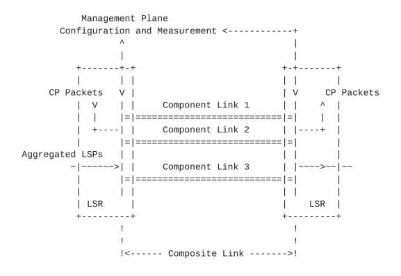
Figure 1 Composite Link Architecture Model
