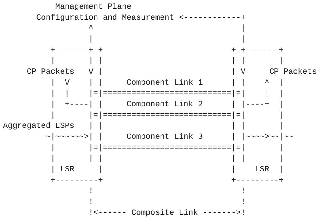
Figure 1 Composite Link Architecture Model
