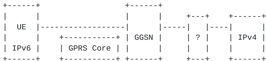
Figure 6: IPv6 node communicating with IPv4 node
