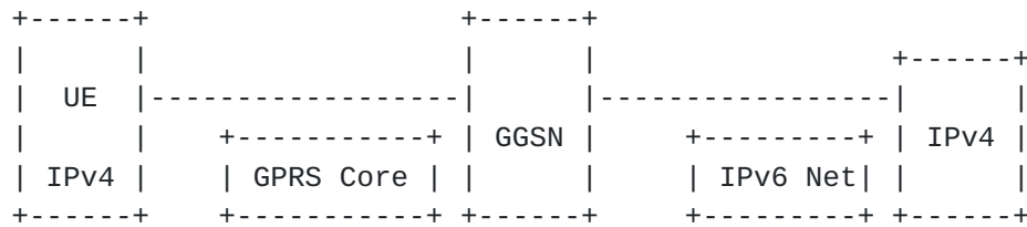
Figure 5: IPv4 nodes communicating over IPv6
