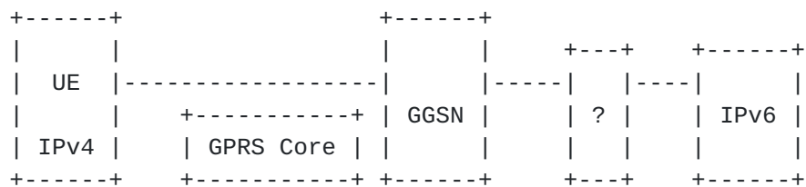
Figure 7: IPv4 node communicating with IPv6 node
