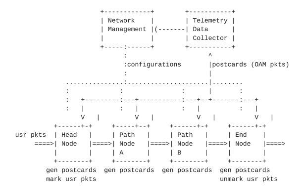
Figure 1: Architecture of PBT-M
