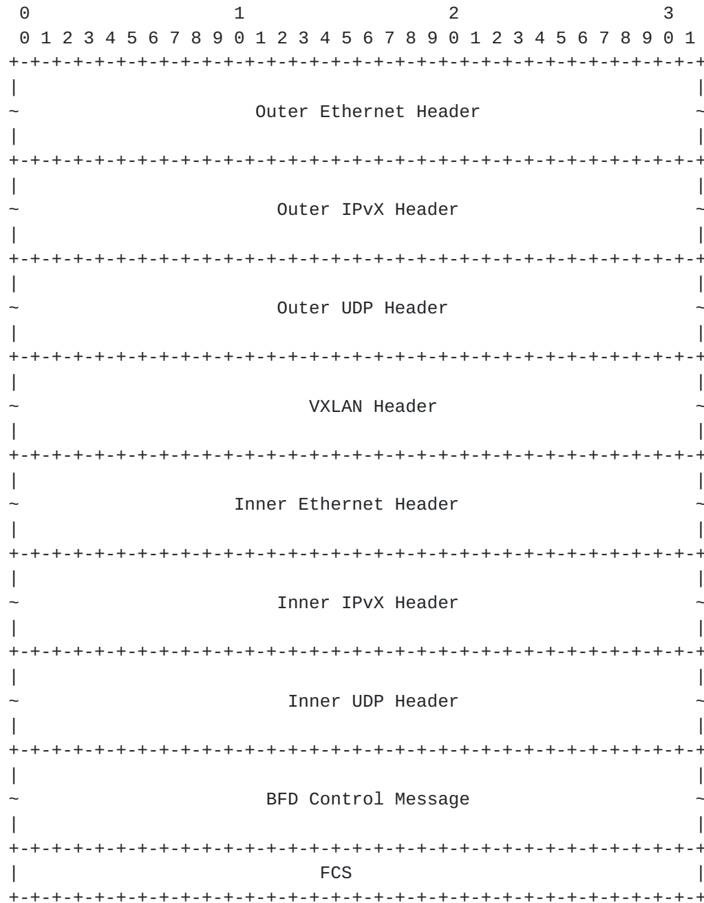
Figure 2: VXLAN Encapsulaion of BFD Control Message
