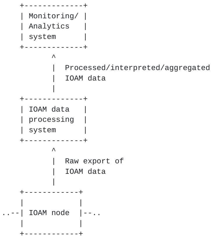
IOAM node: IOAM encapsulating, IOAM decapsulating or
