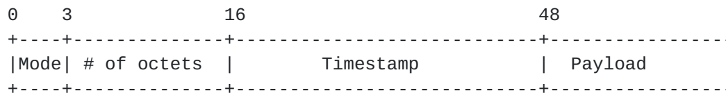
Figure 3: Storage block header structure
