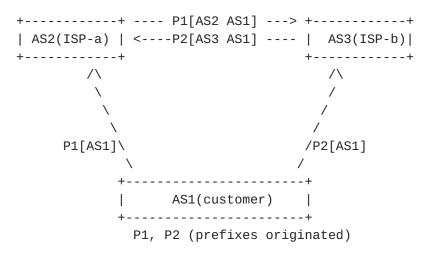
Consider data packet received at AS2 via AS2 or AS3 that originated from AS1 with source address in P1:
