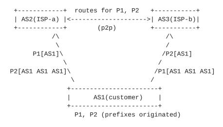
Consider data packet received at AS2 via AS3 that originated from AS1 with source address in P1:
