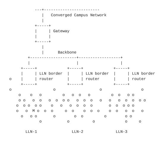
As shown in the diagram, multiple LL Networks are connected to each other via Backbone through LLN Border routers. Each LL Network consist of many nodes. There are different types of traffic forwarded through each LL node and from one LL Network to another. Most LLN traffic types have characteristics similar to that of traditional ones and thus can be supported through existing Diffserv classes except time sensitive control signals. Without segregating
