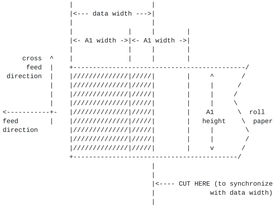
Example 1: "Synchro-Cut", a device cutting the roll paper in synchronization with the data
