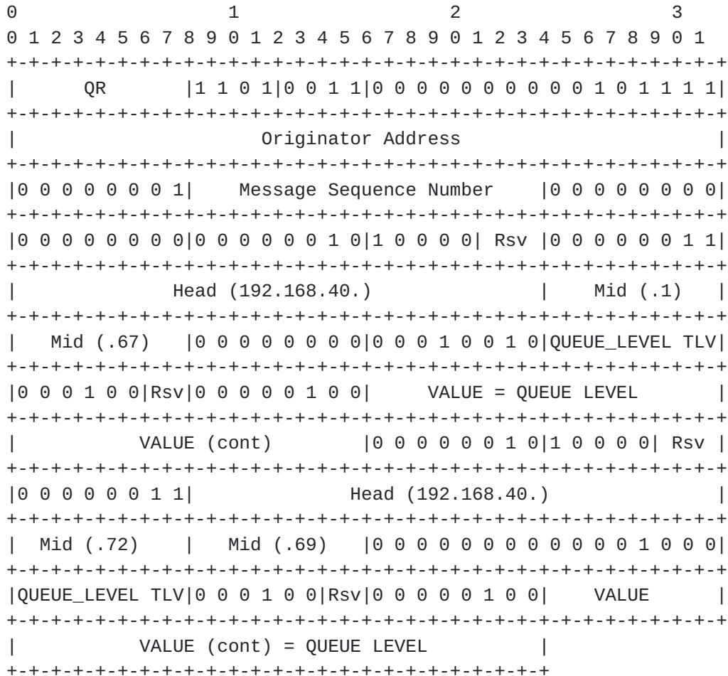
Figure 2: QR Message example of two Flows with a simplified Flow Identifier.
