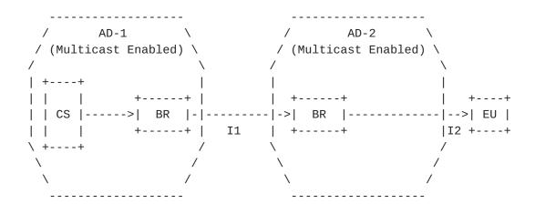
AD = Administrative Domain (Independent Autonomous System) CS = Content Multicast Source BR = Border Router I1 = AD-1 and AD-2 Multicast Interconnection (MBGP or BGMP) I2 = AD-2 and EU Multicast Connection
