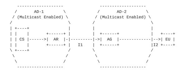
AR = AMT Relay AG = AMT Gateway I1 = AMT Interconnection between P-CDN and S-CDN I2 = S-CDN and EU Multicast Connection
