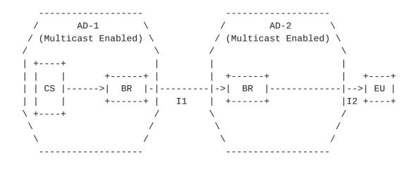
AD = Administrative Domain (Independent Autonomous System) CS = Content Multicast Source BR = Border Router I1 = AD-1 and AD-2 Multicast Interconnection (MBGP or BGMP) I2 = AD-2 and EU Multicast Connection
