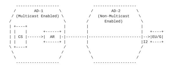
CS = Content Source AR = AMT Relay EU/G = Gateway client embedded in EU device I2 = AMT Tunnel Connecting EU/G to AR in AD-1 through Non-Multicast Enabled AD-2.
