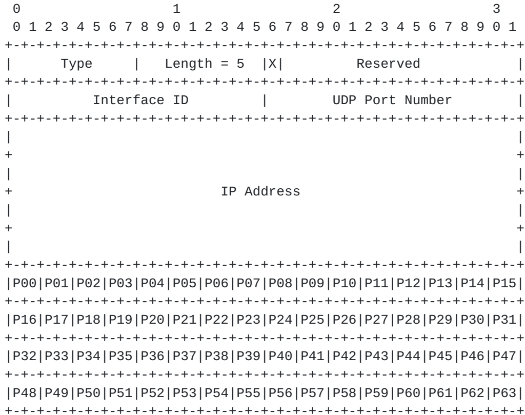
Figure 2: AERO Source/Target Link-Layer Address Option (S/TLLA0) Format
