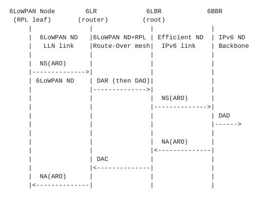
As the network builds up, a node should start as a leaf to join the RPL network, and may later turn into both a RPL-capable router and a 6LR, so as to accept leaf nodes to recursively join the network.
