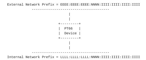
In this figure, L represents the Internal or Local prefix to be translated to the External prefix bits E. The number of L bits is equal to the number of E bits. Subnet bits N and Interface-ID bits I are not changed by the translator.
