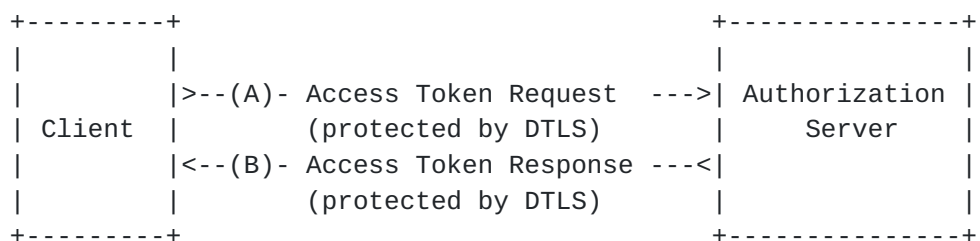
Figure 1: IoT Client Credentials Flow.
